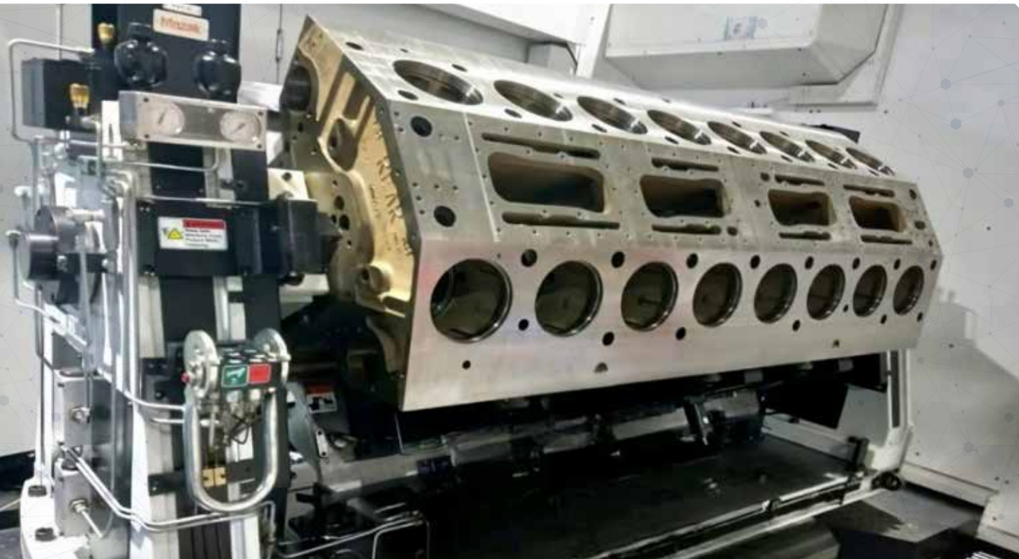
Three position Hydraulic Indexing Fixture, common for 12 and 16 Cylinder blocks. 3-tonne weight, 3.5 m length, and assembly tolerances maintained at 10 microns.
